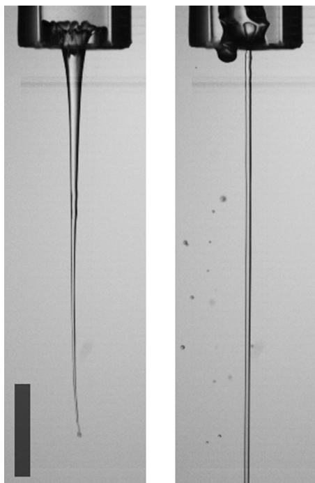
Fig. 11 – Snapshots taken at (a) t = 500 \mu\text{s} and (b) t = 6.5 \text{ ms} from the laser pulse showing (a) tapered jet formation and (b) constant diameter jet. The scale bar is 5 mm.
