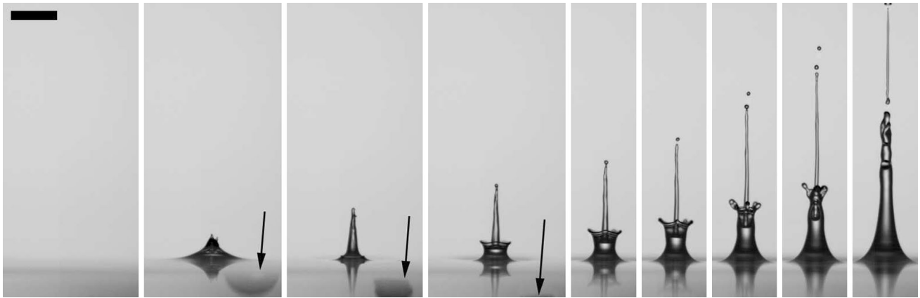
Fig. 3 Example sequence showing the result of a laser pulse focused a few millimeters below the surface. The arrows in frames 2, 3 and 4 indicate the growth and collapse of the cavitation bubble, responsible for the crown formation. Images are taken at times t = -10, 52, 114,
